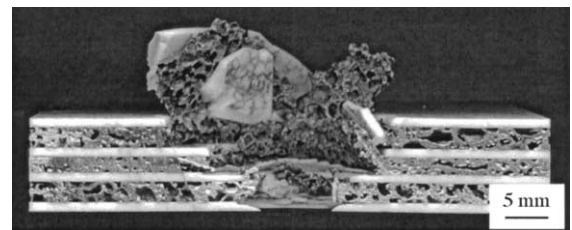
Fig. 16. Cross-section of a penetrated FW/Al 2 O 3 laminate, the surface initially struck by the indenter being at the bottom. Bulging of the rear surface of the target is evident.
