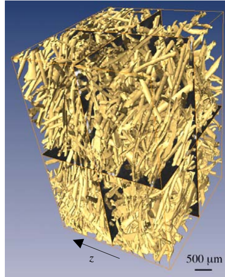
Fig.2: X-ray tomographic image showing 3-D topology of a bonded fibre array. The axial direction ( z ) is also shown.
