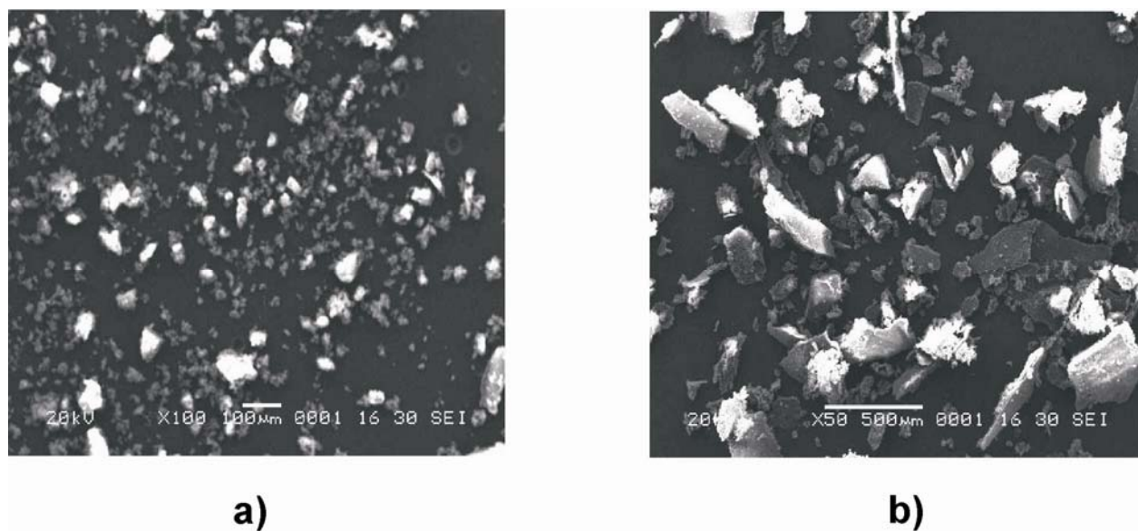
Figure 4. SEM images of ground samples of (phen)(mes). a, a typical sample obtained via neat grinding for 30 min; b, a typical sample obtained via liquid-assisted grinding over a period of 30 min using ethanol as a liquid phase.
