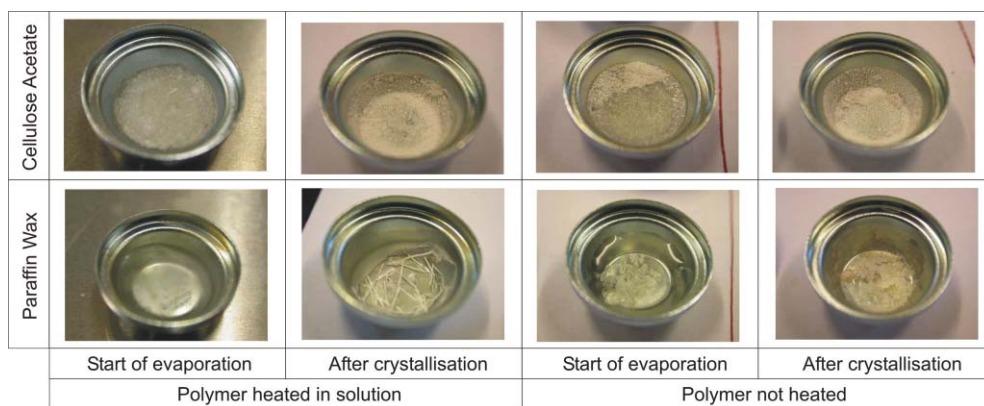
Fig. 6 Photographs showing the appearance of samples containing powders that spread over the surface of the solutions, disrupting the evaporation.
