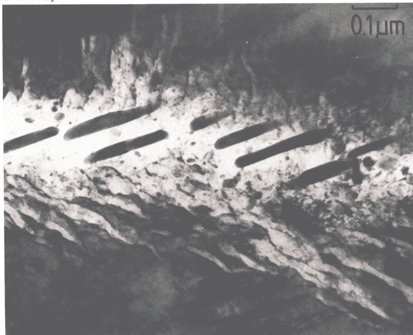
Figure 2 Transmission electron micrograph of lower bainite, whose original interface with the austenite has degenerated into a series of perturbations.
