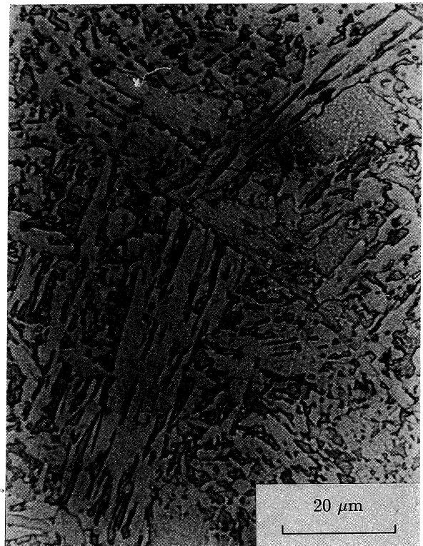
Fig. 6 The bainitic microstructure generated during isothermal transformation at 500°C for 60 min followed by quenching to ambient temperature.
