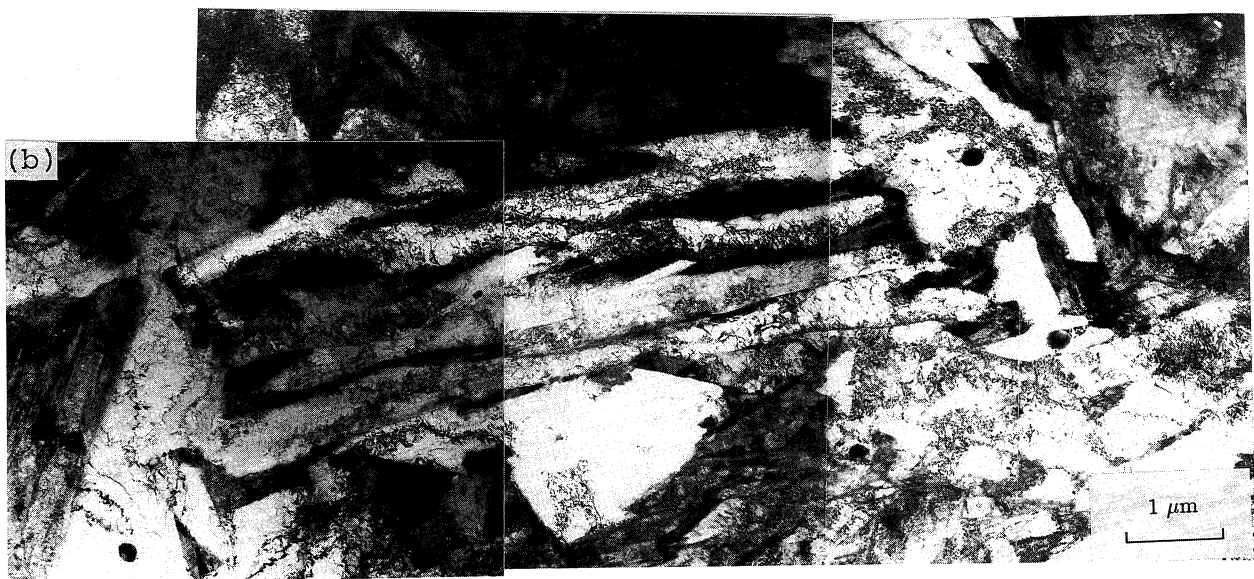
Fig. 8 The microstructure generated by heat-treatment H2, in which the allotriomorphic ferrite is active, with bainite sheaves in the middle of the austenite grains, (a) optical micrograph, (b) thin foil transmission electron micrograph of allotriomorphic ferrite and bainite sheaf.
