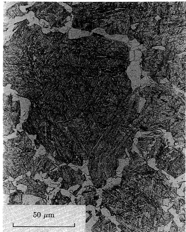
Fig. 10 The microstructure generated by heat-treatment H5, consisting of allotriomorphic ferrite and martensite, since isothermal holding at a temperature above B_s did not cause any transformation.
