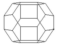
Fig. 5: The shape of the first Brillouin zone for a three–dimensional face centred–cubic lattice.
