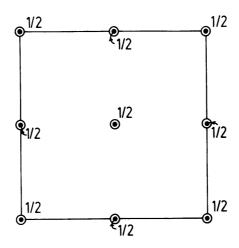
Fig. 9: Projection of the chloride crystal structure along the  $a_3$  axis.
