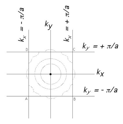
Fig. 4: The first Brillouin zone for a two–dimensional square lattice. Electron energy contours are also plotted. Note the discontinuity at the first Brillouin zone boundary.
