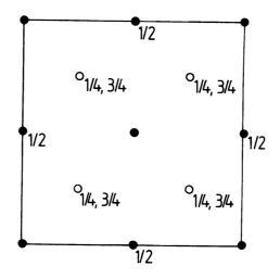
Fig. 10: Projection of the fluorite crystal structure along the  $a_3$  axis.
