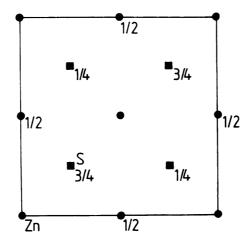
Fig. 8: Projection of the zinc blende crystal structure along the  $\mathbf{a}_3$  axis.
