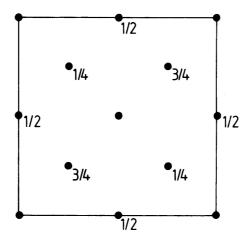
Fig. 7: Projection of the diamond crystal structure along the  $a_3$  axis.
