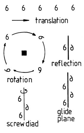
Fig. 6: An illustration of some symmetry operations.
