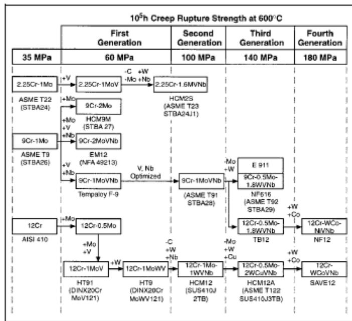
Fig. 1: Evolution of Ferritic Steels for Boilers<sup>[8]</sup>
