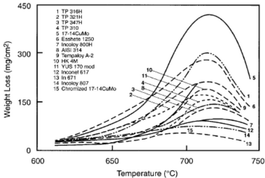
Fig. 6: Comparison of Fire-side Corrosion Resistance of Various Alloys<sup>[13]</sup>
