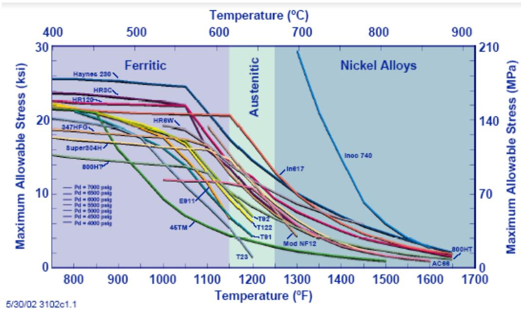
Fig. 4: Boiler Materials for USC Plant(11)
