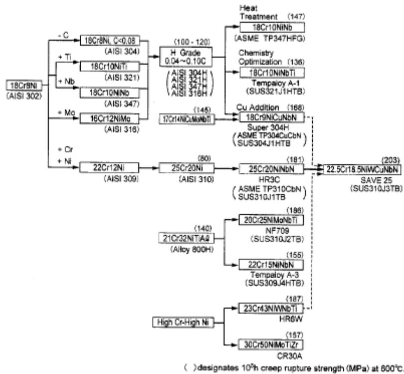
Fig. 2: Development Progress of Austenitic Steels for Boiler (8)
