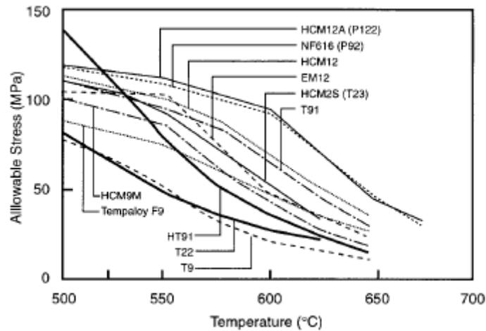
Fig. 3: Comparison of allowable stresses of ferritic steels for boiler (Based on Reference 8)
