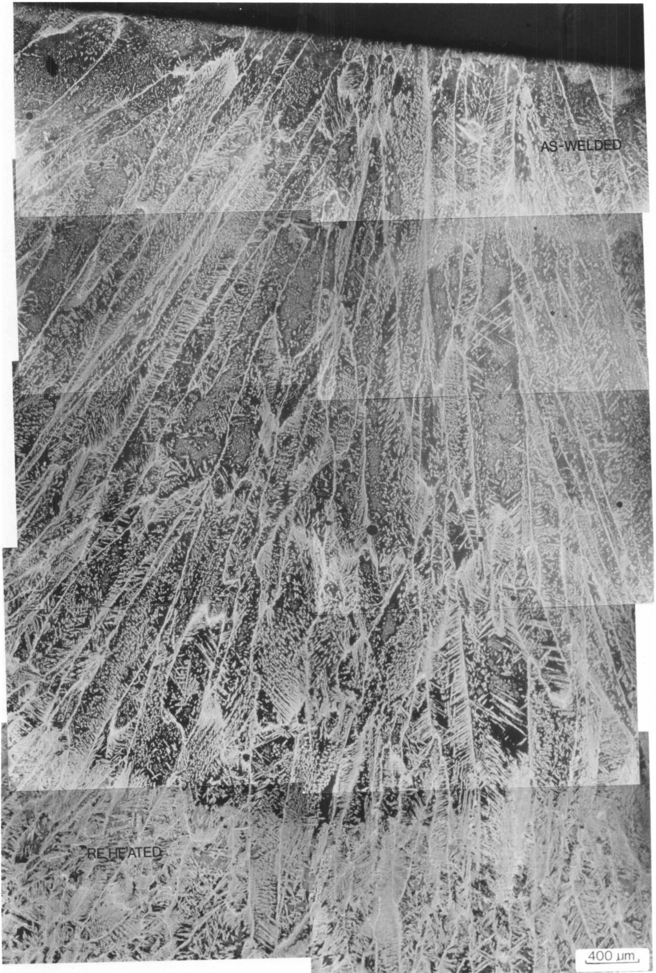
Fig. 3.8: Typical microstructure of duplex stainless steel weld metal,  $\delta$ -ferrite (*dark*), austenite (*light*).
