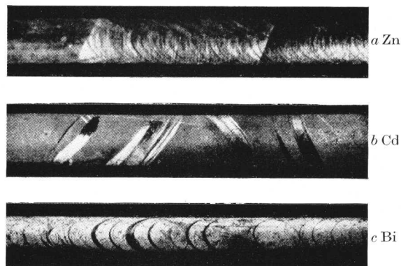
FIG. 48 (a)-(c).—Mechanical Twinning of Metal Crystals.
