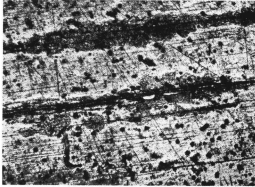
FIG. 147.—Fracture Produced in an Al Crystal by Corrosion Fatigue (294).
