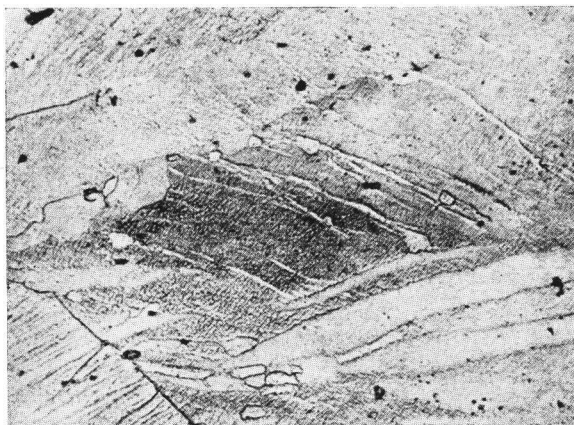
FIG. 162.—Commencement of Recrystallization in the Glide Planes of Low-carbon Steel (402).
