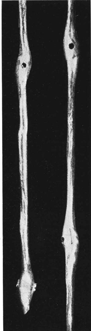
(a) Tensile specimens of a perforated Mg crystal.
