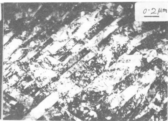
Figure 7(a): Zr-2.5Nb(B); Lath martensite structure
