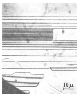
Movement of detwinning along bands in \text{RbNO}_3 . Recrystallization also appearing.
