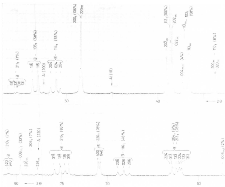
Fig. 2 Room temperature x-ray spectra of Al_4Ca obtained with CoK_{\alpha 1} -radiation
