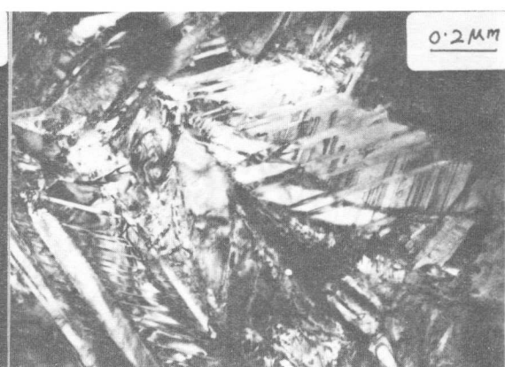
Figure 8(a): Zr-5.5Nb(B); Internally twinned plate martensite
