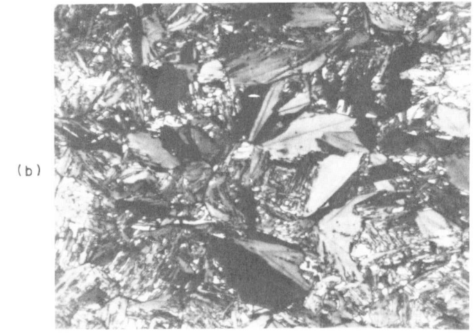
FIG. 7 Field-induced morphological transition in Fe-29.6Ni at -2^{\circ}\text{C} . (a) Laths at 40 kOe, (b) mixture of plates and laths at 140 kOe.
