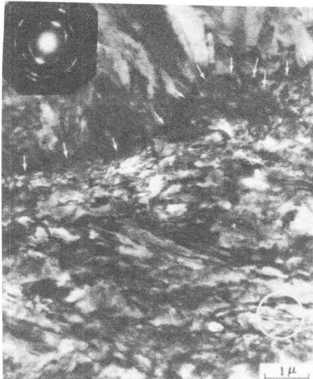
Fig. 1 Profile TEM fractograph and diffraction pattern in 9Ni steel. The fracture surface (indicated with arrows) was plated with iron (above the boundary indicated with arrows) to prepare thin foils of the fracture surface layer. The diffraction pattern was taken from the central region right below the boundary line. The circled area shows \gamma_R -like particles which have transformed to \alpha' .
