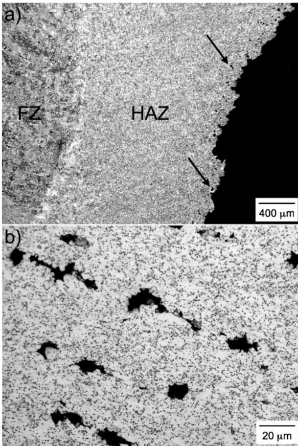
4 Optical micrographs obtained from ruptured specimens showing *a* localised formation of creep voids in fine grained HAZ beside fracture surface in sample 5 and *b* creep voids beside fracture surface in sample 8 at higher magnification: in *a*, FZ denotes fusion zone; loading direction was from left to right in both images
