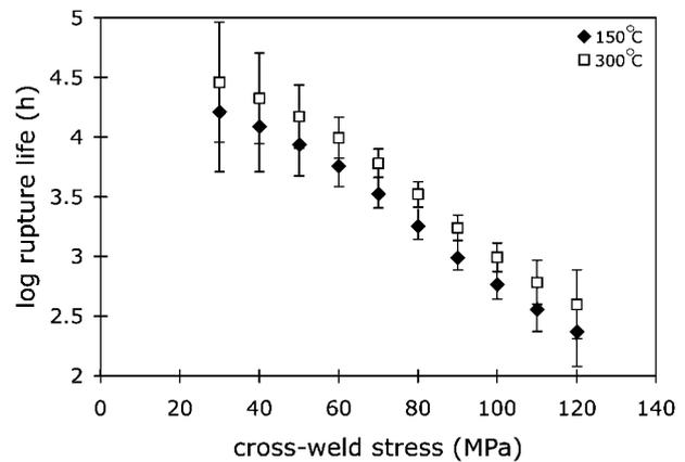
7 Neural network predictions for type IV limited rupture life in cross-weld test on P91 steel at 620°C: influence of stress is shown for two different preheat temperatures, joint preparation angle of 30° and heat input of 1.6 kJ mm<sup>-1</sup>
