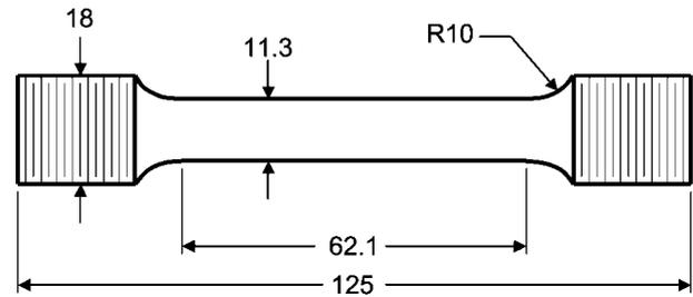
**3 Configuration of creep test specimens in current work: all dimensions are given in mm**
