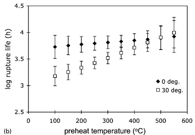
5 Neural network predictions for type IV limited rupture life in cross-weld test on P91 steel at 620°C and with stress of 80 MPa showing *a* influence of joint preparation angle with two different preheat temperatures and *b* influence of preheat temperature using two different joint preparation angles: weld heat input was  $1.6 \text{ kJ mm}^{-1}$
