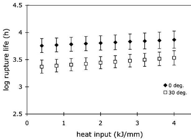
6 Neural network predictions for type IV limited rupture life in cross-weld test on P91 steel at 620°C and with stress of 80 MPa: influence of weld heat input is shown for two different joint preparation angles and preheat temperature of 250°C
