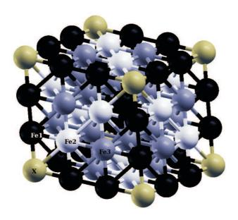
FIG. 1. (Color online) The model of  $3 \times 3 \times 3$  supercell of the primitive cell of bcc Fe, which contains 27 atoms. The Fe1, Fe2, and Fe3 atoms are represented by black, white, and grey spheres, respectively, while the impurity atom (corner atom) is marked with X.
