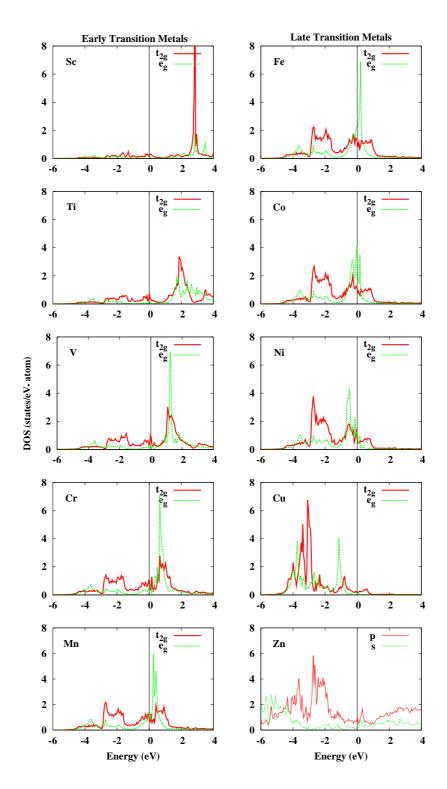
FIG. 3. (Color online) Calculated spin-unpolarized impurity-atom-projected local density of states of  $X_1$ Fe<sub>26</sub>. Solid (dotted) lines represent the  $t_{2g}$  ( $e_g$ ) states, whereas the thin solid (dotted) lines show the s(p) states, which are multiplied by a factor 20, of Zn impurity at the left bottom. First (second) column shows early (late) transition metals. The Fermi energy ( $E_F$ ) is set to zero.
