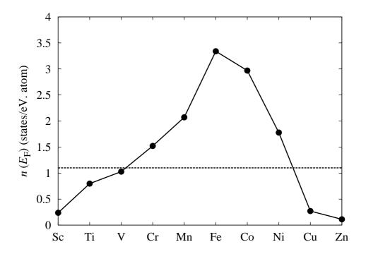
FIG. 4. Calculated local density of states at the Fermi energy,  $n(E_{\rm F})$ , for the 3d impurities in nonmagnetic bcc Fe. The dotted horizontal line represents the Stoner limits for the local spin-polarization.
