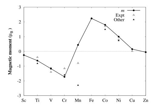
FIG. 5. Calculated local magnetic moment of the 3d impurities in bcc Fe. Filled circles show our calculated local magnetic moment (in units of  $\mu_{\rm B}$ ) at the X site, filled triangles show the previously calculated values (Other),<sup>8</sup> and open triangles show the experimental (Expt.) values taken from Refs. 20, 26–31.
