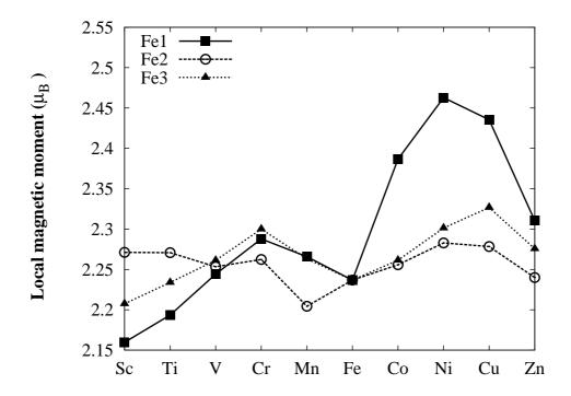
FIG. 7. Calculated local magnetic moments (in units of  $\mu_{\rm B}$ ) of Fe1, Fe2, and Fe3 atoms. Filled squares and triangles represent the local magnetic moments of Fe1 and Fe3 atoms, respectively, whereas the open circles represent Fe2 atoms.
