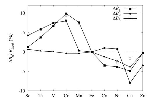
FIG. 11. Calculated Fermi contact hyperfine field changes  $\Delta B_n$  normalized by the host Fermi contact hyperfine field  $B_{\text{host}}$  in the 1st, 2nd and 3rd shell around the 3d impurities in bcc Fe. Here n represents the 1st, 2nd, and 3rd Fe atoms. The filled squares, triangles, and circles represent  $\Delta B_1$ ,  $\Delta B_3$ , and  $\Delta B_2$  respectively, whereas open symbols represent the experimental values taken from Ref. 50.
