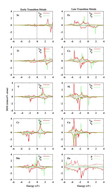
FIG. 8. (Color online) Calculated spin-polarized impurity-site-projected local density of states of  $X_1$ Fe<sub>26</sub>. The upper (lower) panels show majority (minority) spin states. Solid (dotted) lines show the  $t_{2g}$  ( $e_g$ ) states, whereas for the Zn impurity at the left bottom the thin solid and dotted lines show the s and p states, which are multiplied by a factor 20. First (second) column shows early (late) transition metals. The Fermi levels ( $E_F$ ) are set to zero.
