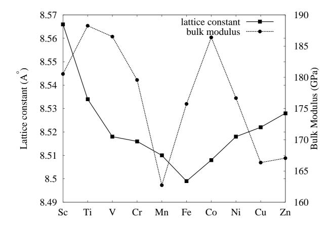
FIG. 2. Calculated optimized lattice constant a (in units of Å) and bulk modulus B (in units of GPa) of  $X_1$ Fe<sub>26</sub>. Filled squares (circles) on the left (right) axis show lattice constant (bulk modulus).
