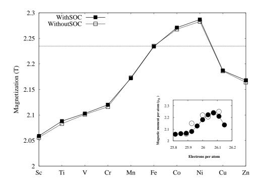
FIG. 6. Calculated total magnetization M of  $X_1\mathrm{Fe}_{26}$  (in units of T). Open squares show M without spinorbit coupling (SOC) and filled squares show M with SOC. The horizontal dotted line shows M of pure Fe without SOC. The inset shows the atom averaged magnetic moment  $(\bar{m})$  (open circles) in units of  $\mu_{\mathrm{B}}$ without SOC versus the number of electrons per atom of  $X_1\mathrm{Fe}_{26}$ . The filled circles show the experimental values taken from Ref. 44.
