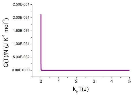
Fig. 23. The specific heat of the cell gas model of Fe<sub>2</sub>MnAlC  $\kappa$ -carbide
