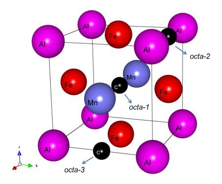
Fig. 10. Octa-1, Octa-2, and Octa-3 position of carbon in Fe<sub>2</sub>MnAlC κ-carbide unit cell.
