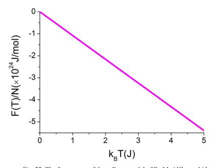
Fig. 22. The free energy of the cell gas model of Fe<sub>2</sub>MnAlC  $\kappa$ -carbide
