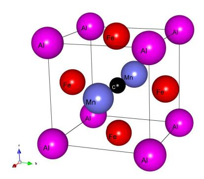
Fig. 9. The structure of Fe<sub>2</sub>MnAlC  $\kappa$ -carbide
