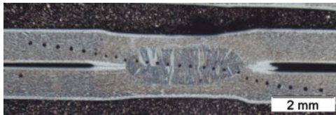
9 Hardness measurement across weld nugget
