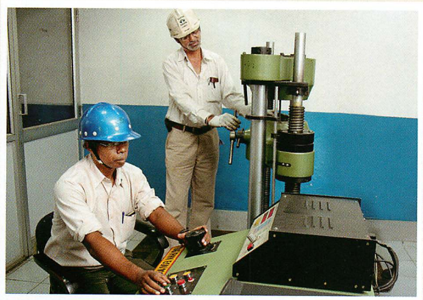
Compression testing machine in the Physical Laboratory
