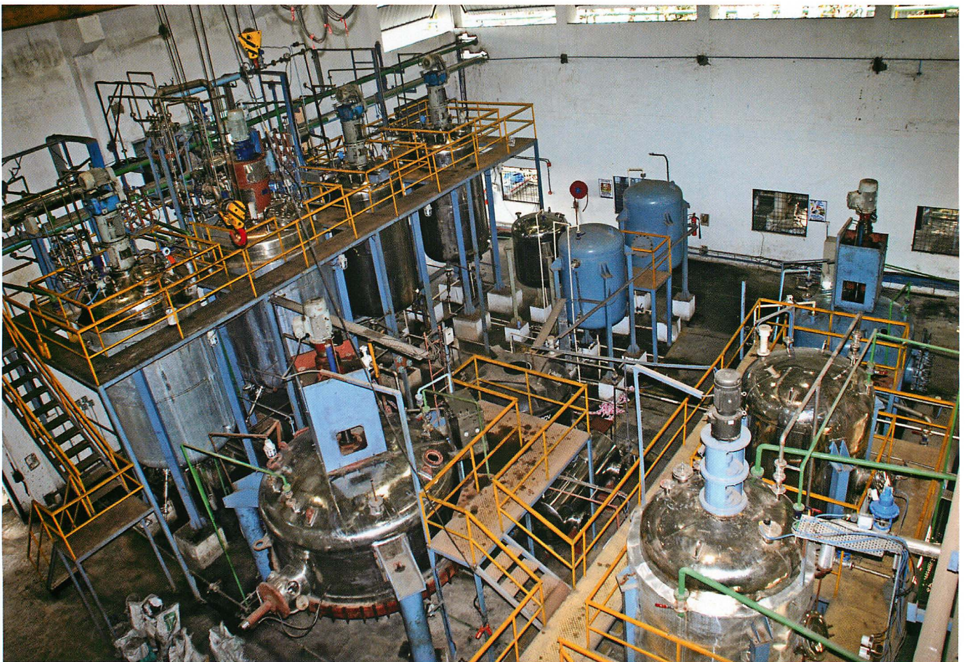
Semicontinuous pilot plant for chemical beneficiation of coal (2011)
