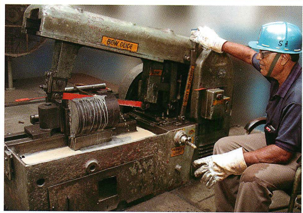
Power Saw for sample cutting at the Physical Laboratory
