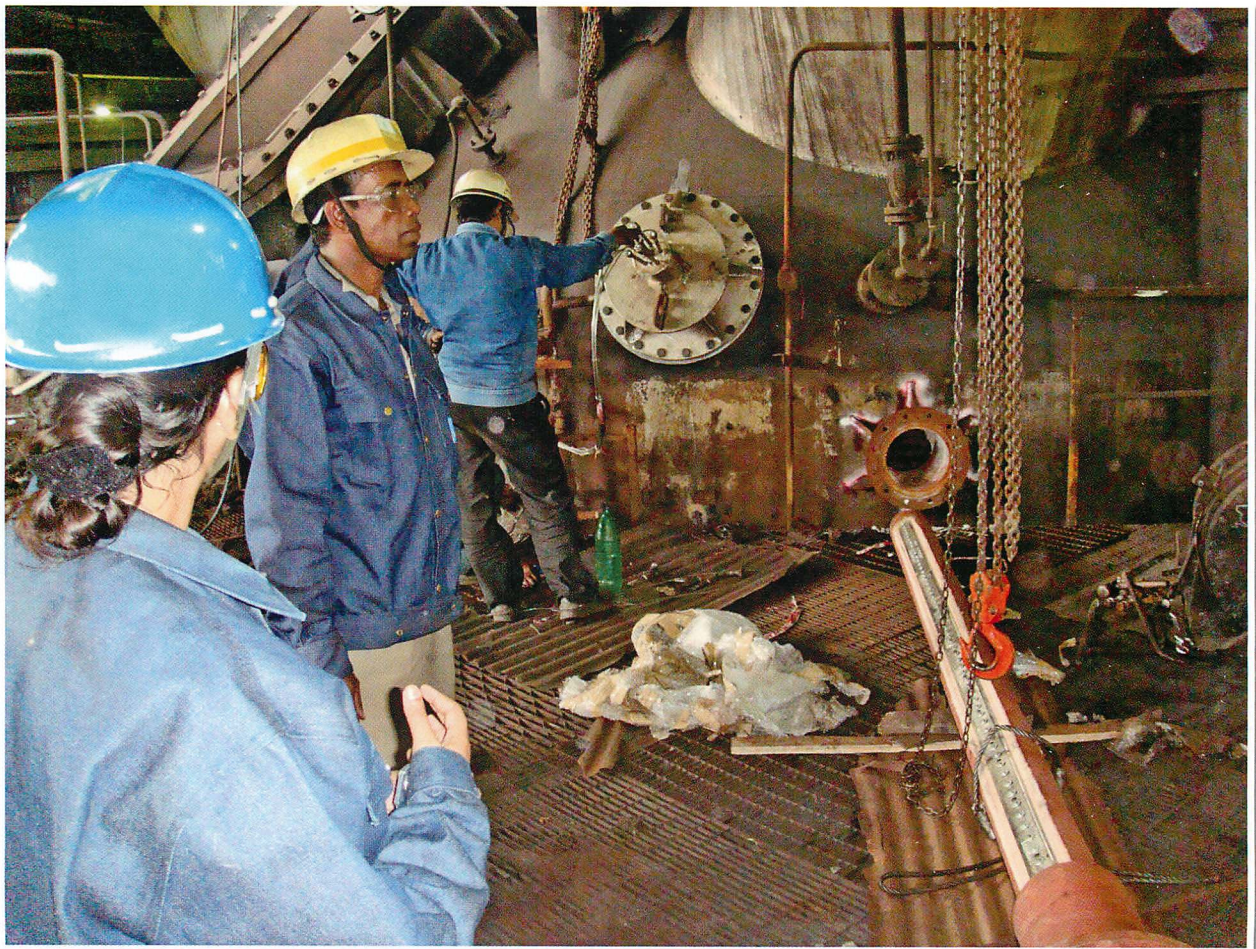
Probing the Blast Furnace using an advanced material trajectory probe (2010)
