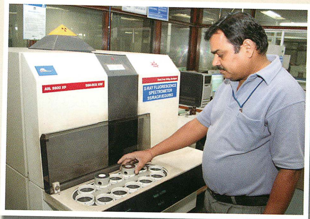
X-Ray Fluorescence Spectrometer in Chemical Laboratories
