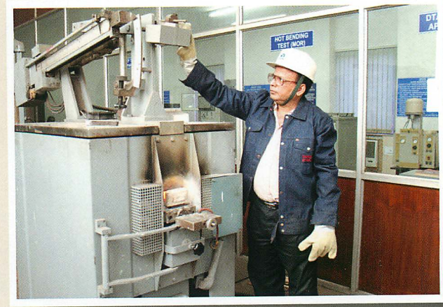
Hot Modulus of Rupture H-MUR
