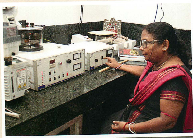
Carbon coating unit in the Metallography lab
