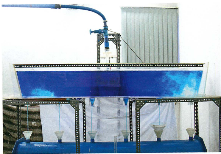
Scaled down water model of the billet caster tundish at Tata Steel
