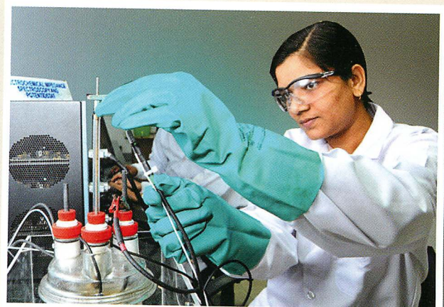
Electrochemical Impedance Spectroscopy facility in the Advanced Corrosion Laboratory
