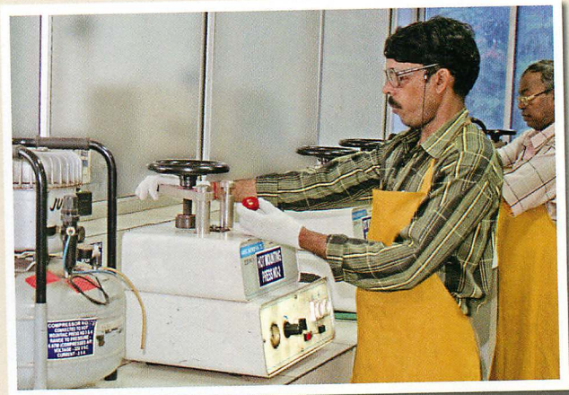
Hot mounting press in the Metallography Laboratory
