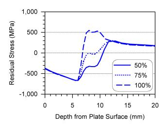
Figure 11: Effect of final austenite fraction on the predicted stress when the interpass temperature is kept at  $50^{\circ}$ C.
