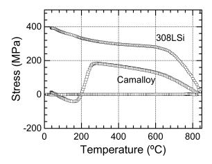
Figure 1: a) Stress recorded during constrained cooling (Satoh test) of the two filler metals used in this study [12]
