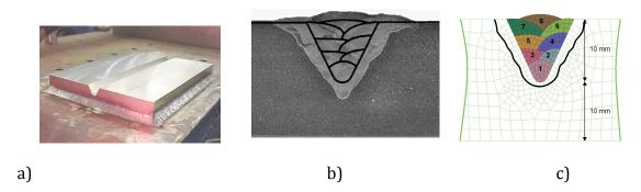
Figure 2: a) A photograph of the grooved plates prepped for welding b) optical macrograph showing the fusion zone and the weld lay-up sequence for the gas metal arc welds, c) finite element mesh used in the multipass weld model showing each pass and the  $1500^{\circ}$ C thermal contour that approximates to the fusion zone boundary.
