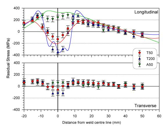
Figure 6: Longitudinal (top) and transverse (bottom) residual stress profiles as a function of distance from the weld centrelines at a depth of 4mm below the plate surface. Markers denote neutron diffraction measurements and the corresponding solid lines denote the contour method results for the same plate.
