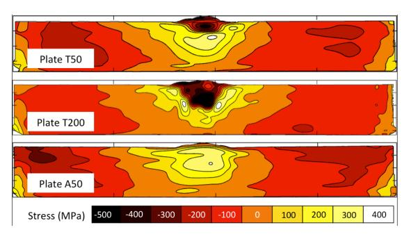
Figure 7: Maps of longitudinal residual stress calculated using the contour method for plates T50, T200 (both Camalloy 4) and A50 (308L).
