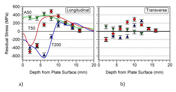
Figure 5: a) Longitudinal and b) transverse residual stress profiles with depth through the thickness of the plates at the weld-centreline. The markers denote neutron diffraction measurements while in (a) the corresponding continuous lines denote the contour method results for the same plate.
