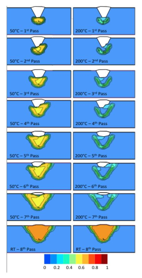
Figure 8: The predicted martensite fraction for after the laying down of each pass for interpass hold temperatures of  $50^{\circ}$ C (left) and  $200^{\circ}$ C (right). After the  $8^{th}$  pass the plate has been allowed to cool to room temperature.
