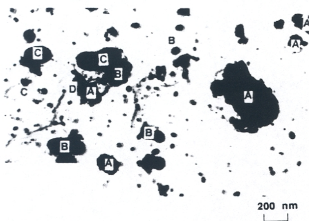
Fig. 2 Particles for the as-received specimen in a carbon extraction replica. Relative atomic percent ratio for the metallic elements in the marked particles are
