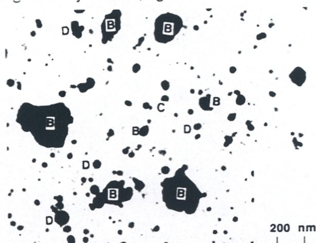
Fig. 3 Particles in a carbon extraction replica from the continuous heating experiment, at 1230 °C recrystallised and water quenched. Relative atomic percent ratio for the metallic elements in the marked particles are
