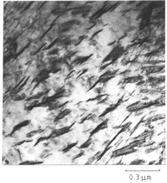
Figure I.10e Morphology of lower bainitic cementite.
