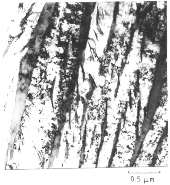
Figure I.6 Upper bainite formed after isothermal transformation at 350°C for 205 min. The retained austenite is the grey phase.
