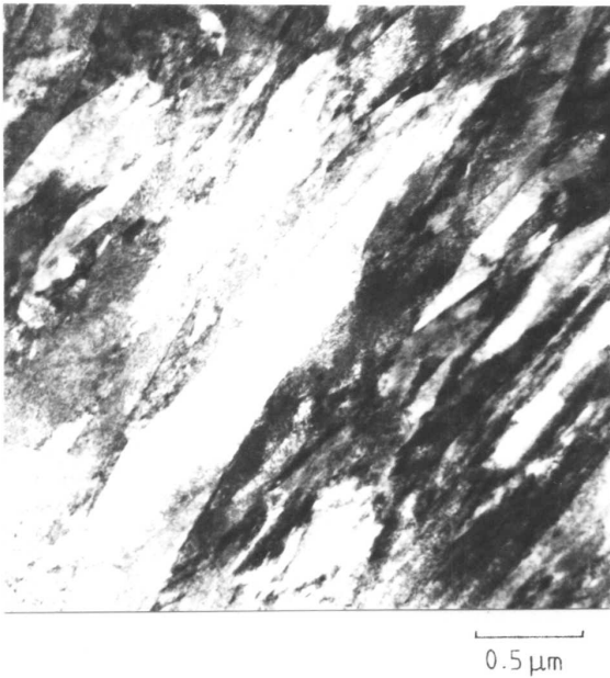
Figure I.11 Typical microstructure of lath martensite resulting from a direct quench following austenitisation.
