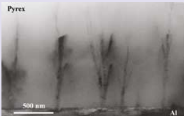
Transmission-electron micrograph of dendritic nanocrystalline \gamma -alumina structures at an anodically bonded Pyrex-Al interface
