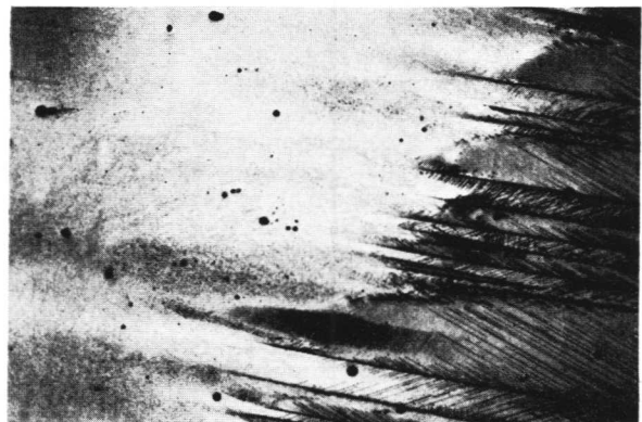
Fig. 6 Transition zone between the cubic structure and the twinned tetragonal structure in a single crystal of AuCu quenched after partial transformation in a temperature gradient. 41 \times 50 .
