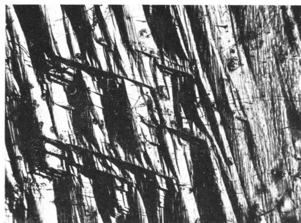
Fig. 1 Surface-relief effects associated with plates of \gamma -Hg on two variants of the \{\bar{1}13\} habit plane. \times 80 .
