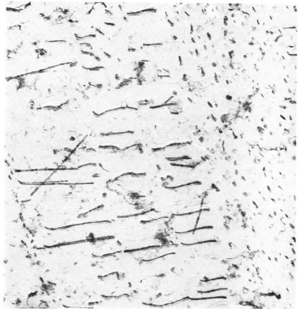
Fig. D.VI.7 Carbon replica of Fe-0.5% V-0.1% C steel transformed at 840^\circ C , showing rods. \times 15,000 . (Collins.)
