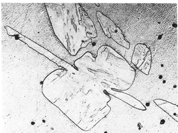
Fig. 8 Micrograph of a 14.6% Cr alloy. Initial structure ferrite. Anneal 2 h at 950° C (( \alpha + \gamma ) range), water-quench. \times 320 .
