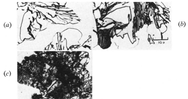
Fig. 1 Showing increasing tendency for co-operative growth with increasing undercooling: (a) 581° C, 90 min; (b) 574° C, 40 min; (c) 556° C, 8 min (partially transformed specimens of Fe–2.3N).
