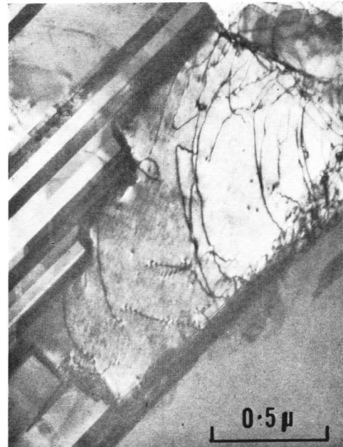
Fig. 3 Twinned areas in the \alpha_m phase showing micro-twins associated with the steps on the boundary of the larger twin.
