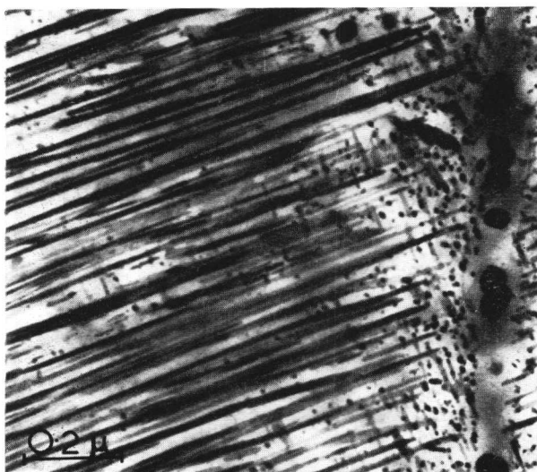
Fig. 2. Fe-4Mo-0.2C alloy isothermally transformed for 30 min at 700° C. Thin-foil electron micrograph. \times 68,000 .
