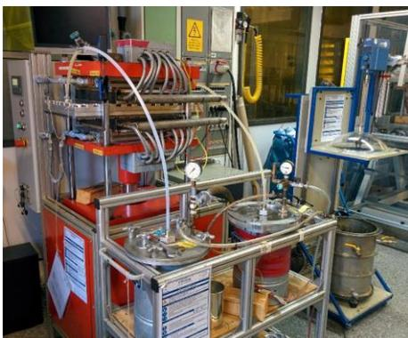
RTM (Resin Transfer Mould) press
