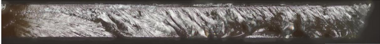
Fatigue fracture surface. A glass fibre is visible along the top edge.
