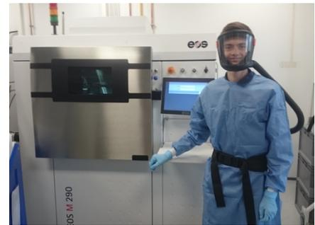
Me being introduced to the main printer. The safety gear protects your lungs from breathing in the small metal particles.
