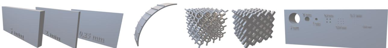
From left to right: vertical walls with thickness labels, a curved overhang with bars every 10°, a diamond type lattice, a lattice with only 45° overhangs, and a wall with lateral holes (labels give the radius of the hole).
