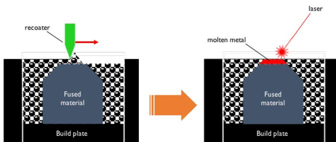
Powder deposition (left) and laser melting (right). These two steps are repeated until the part is complete.
