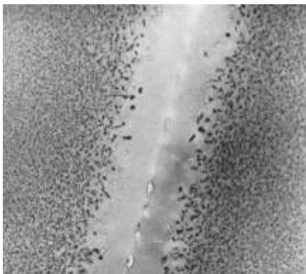
A grain-boundary precipitate-free zone [Unwin, Lorimer & Nicholson (1969)]
