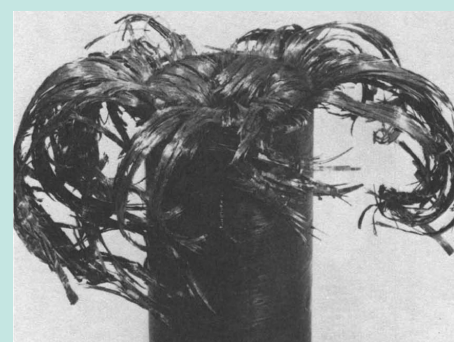
Progressive crushing of fibre-reinforced composite tubes [D Hull (1991)]
